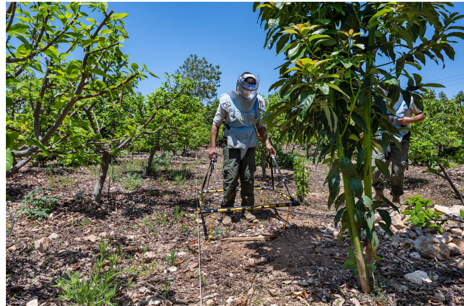
© 2023, Arne Hodalič/ITF Enhancing Human Security | A clearance operator from Norwegian People's Aid (NPA) uses a large-loop detector to search for cluster munition remnants in an orange orchard in Al Makiyeh in Lebanon's South governorate.
