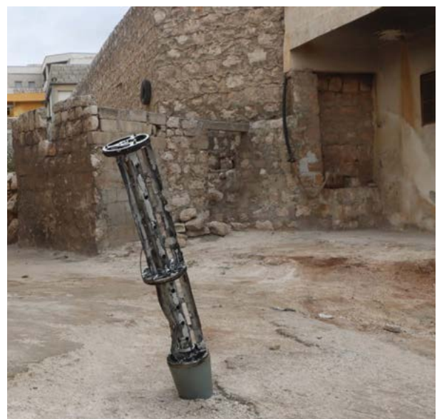
The empty cargo section of a fired cluster munition rocket in the city of Darat Izza, in Syria's Aleppo governorate.
