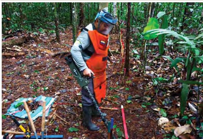
A deminer from the Colombian Campaign to Ban Landmines (CCCM) uses a metal detector to locate landmines in the Cumaribo municipality of Vichada department, in Colombia.
