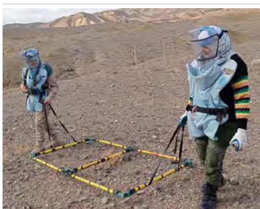
A Fondation Suisse de Déminage (FSD) demining team uses a large loop detector to scan for explosive remnants of war during clearance operations in Shurob, Tajikistan.
